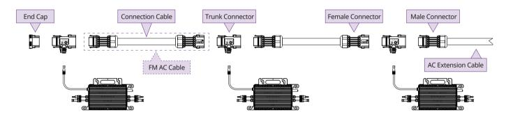
\* Using Plug and Play Cable: VaySunic offers various FM AC Cable lengths including 2.2m. If you require a different length, contact VaySunic GmbH.
