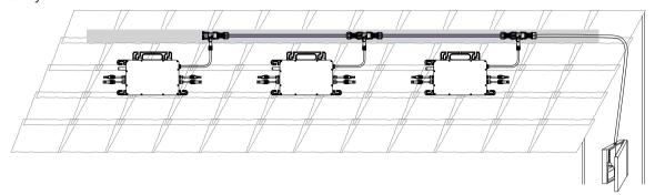
The AC output line consists of five main components: End Cap, Trunk Connector, Female Connector, Male Connector and Connection Cable.
